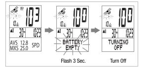
When the power is less than 10%, the low battery indicator will flash every 60 seconds. The battery needs to be recharged.
