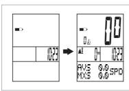
Auto Wake Up: When there is any speed or vibration, the computer will wake up
