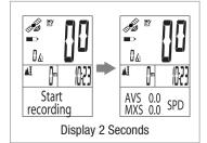
Press RECORD button to stop recording. Press MODE button to select Yes. Press RECORD button to select No and continue riding.
